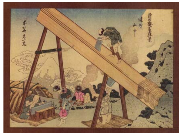
Timber-Handling Technology in Japan. Fig. 2 Sawyers rip a squared timber at Yamanaka in Tōtōmi Province, southwest of Mt Fuji, while another workman, seated before their temporary mountain hut, sharpens his saw, as family members look on. (Katsushika Hokusai, Thirty Six Views of Mt. Fuji (ca. 1820), in the author's possession.)
